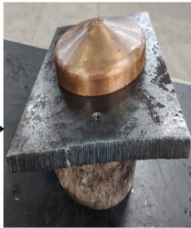
Copper Lance Head mounted on Fixture
