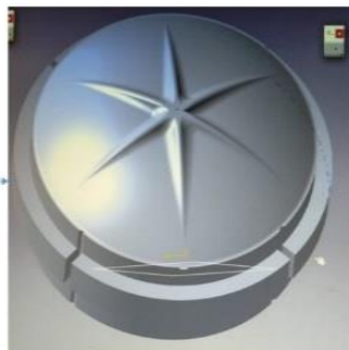
CAD Model prepared by reverse engineering
