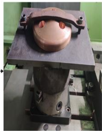
Copper Lance Head mounted on Fixture while machining
